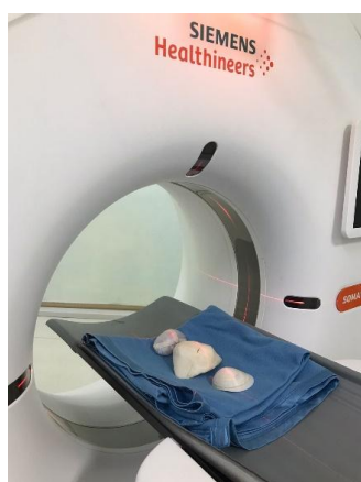
Figure 2. Sample irradiation with CT-Scan
