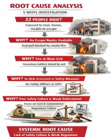
Figure 2. RCA Fire in Terra Drone Building
