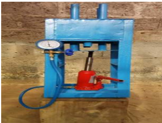
Manually fabricated handpress (Aliyu, et al., 2021)
