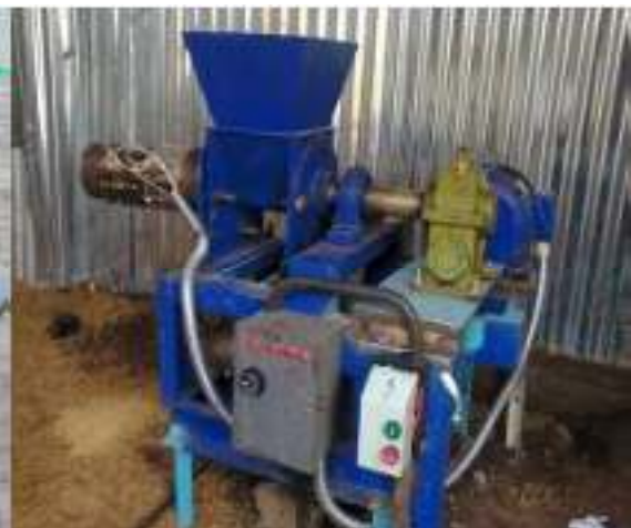
Mechanical co-centric screw press (CTCT, 2020 )
