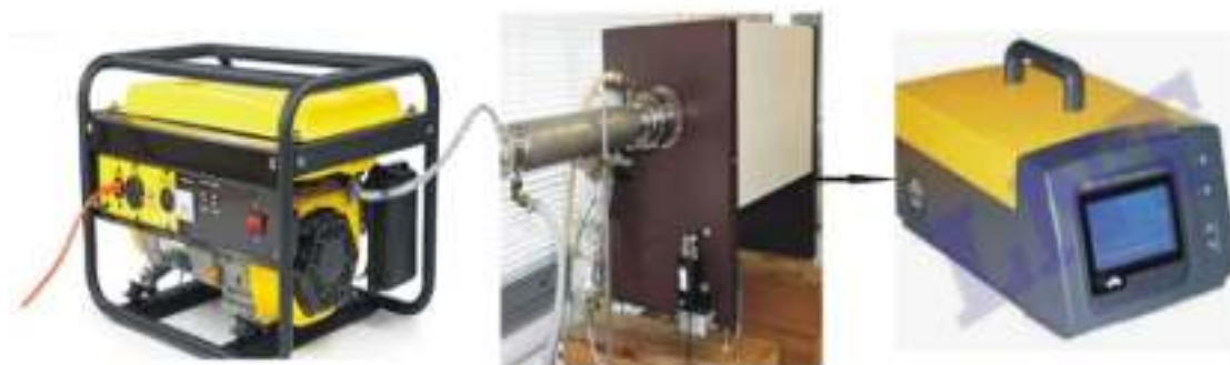
Figure 1. Testing of synthesized MOF using Gas Analyzer
