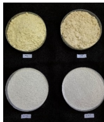
Fig 2. The photograph of soybean flour/SF (top left), tempe flour/TF (top right), soybean protein concentrate/SPC (bottom left), tempe protein concentrate TPC (bottom right)
