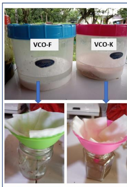
Figure 4. The VCO extraction by a fermentation process using moringa leaf (VCO-K) and yeast (VCO-F)
